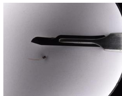
Figure 8. Locator screw fragment
