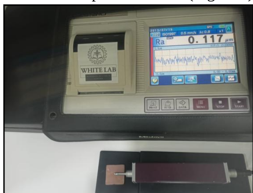
Figure 3. Recording of Surface Roughness using a Profilometer
