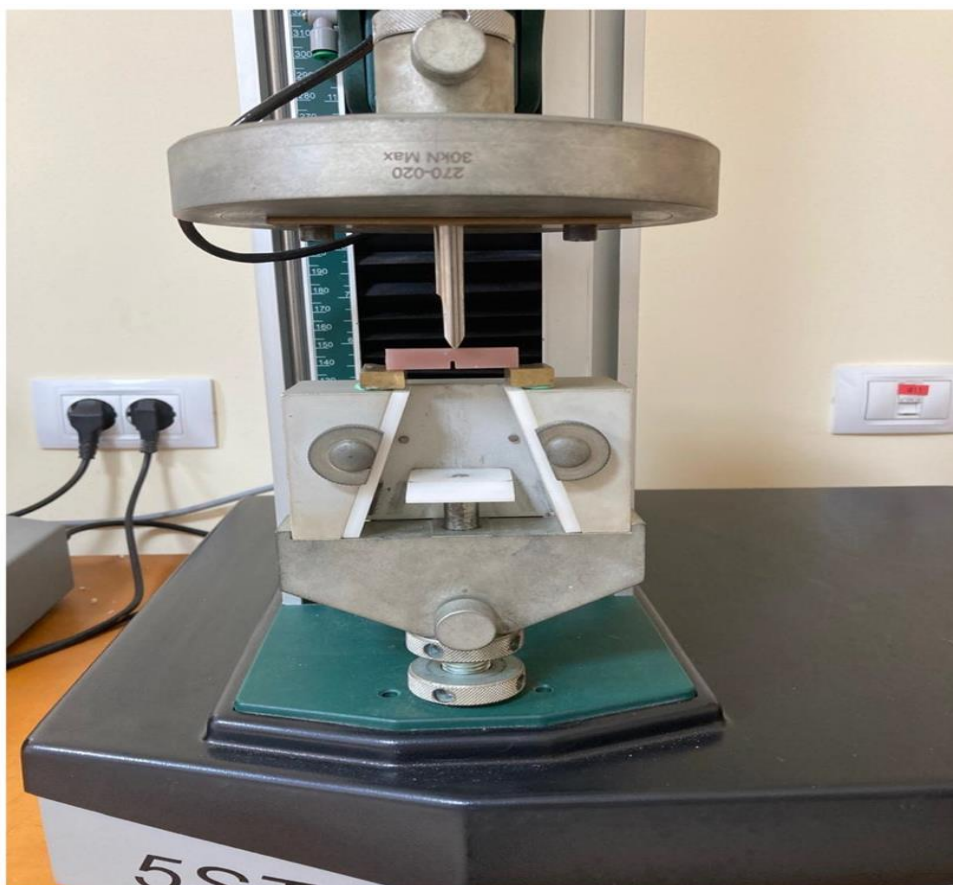
Figure. 2 Photograph of the fracture toughness test.
