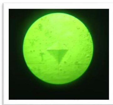
Figure 1. (Photomicrograph of an indentation made with the hardness tester)
